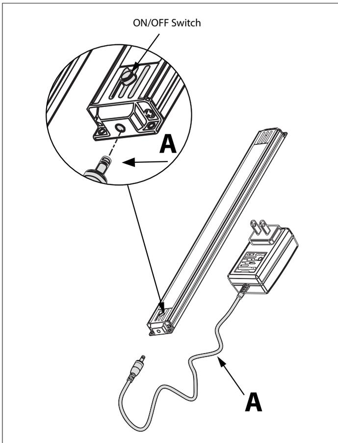
**2** Use connector cords (B) to connect additional lights. Up to 4 LED lights can be connected to one Power adapter cord (A).
