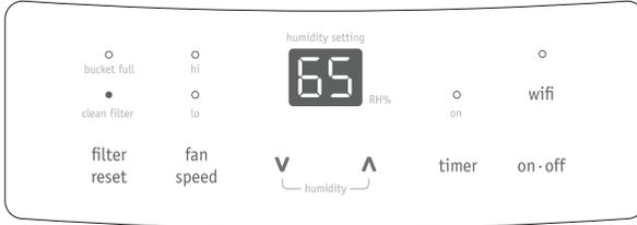
6. The TIMER function enables you to either Delay Start or Delay Stop the unit in the choice from 0.5 hour to 24 hours. If the unit is running, then selecting Timer will turn the unit off in the hours that will be set (Delay Stop). If the unit is off, then selecting Timer will turn the unit on in the hours that will be set (Delay Start).
