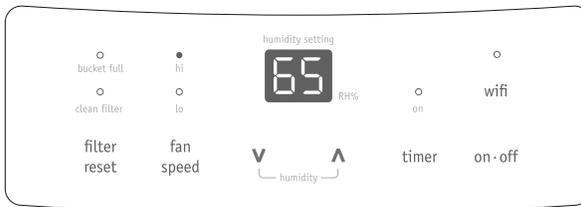
4. You can also use the FAN SPEED button to change the fan speed to HIGH or LOW. The indicator light will show the setting you have selected. A higher fan speed will result in quicker moisture removal.
