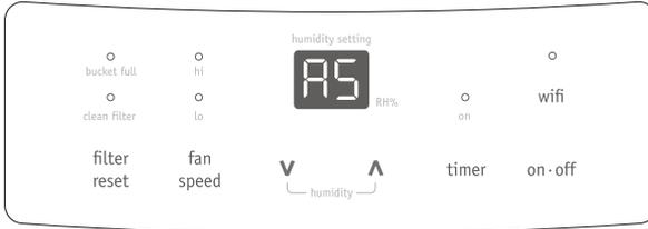
2. If the display reads "EC", check the following operating conditions. Outlet voltage should be 115V±10% and the surrounding temperature should be with in the range of 41 °F to 96 °F. Unplug the unit and plug it in again under normal operating conditions. If the "EC" code persists, contact your Authorized Frigidaire Service Center.
