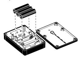
Replace the cover making sure the perimeter seal (O-ring) is in place, then securely tighten the six (6) screws. Be sure not to over-tighten screws.
