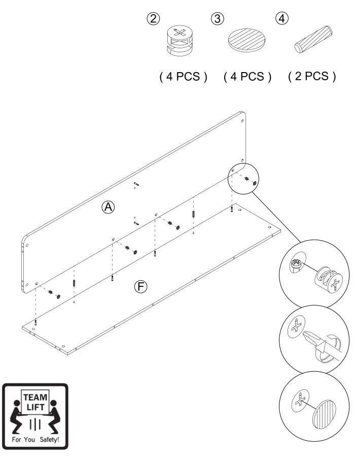
\* Attach the TOP (A) to the MEDIAN PANEL (E) by the Two KD CAM (2) , Two COVER CAP (3) ,and Eight WOOD DOWEL (4) .
