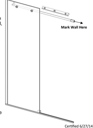
**9** After marking, remove header assembly [8]. Drill a 1/4" diameter hole approximately 1 3/4" deep, at the marked wall location.
