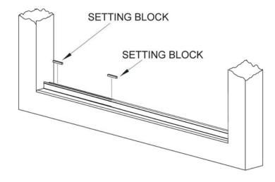
**7** Using suction cups, set the Glass Panel into the U-channels on the appropriate side. Use different sizes of setting blocks to make exposed edges of the glass level and plumb.\*\*
