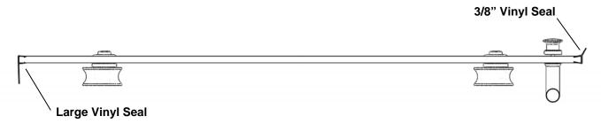
**16** The larger vinyl seal will need to be cut slightly in order for the header bar to have space to roll freely. See example below.
