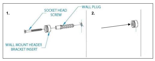
**10** Reassemble the roller bar header assembly [8] by securing the header assembly to the wall mount header bracket and then tightening down the set screws.
