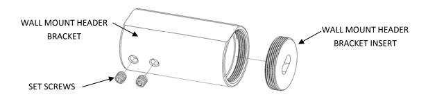
Next, put the supplied large wall plugs into the hole. Screw the inner part of the Header Bracket into the wall with the supplied socket countersunk head screw.
