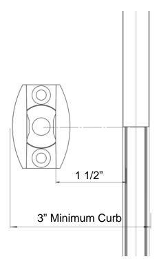
**Note**: Centerline (CL) is a term used to describe the center or mid-point of the unit. The position of the unit centerline can be located anywhere within the width of the threshold, as long as adequate structure exists beneath the centerline for fastening and the outer edges of the unit will not overhang the threshold. The most common unit centerline position is the middle of the threshold.
