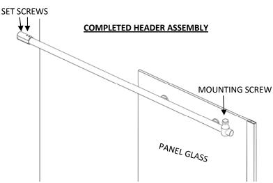
NOTE: Flat side of wall mount header bracket should face towards the door. Do not over-tighten screws.
