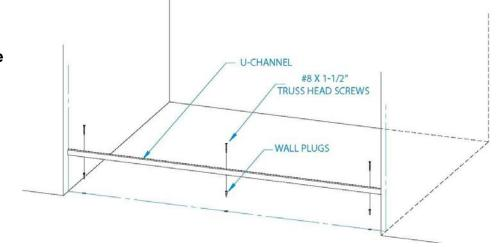
**3** Insert a small amount of silicon into each drilled hole, then insert a wall anchor into each hole. (Note: Drill hole, then insert a wall anchor.) This must be done just before u-channel installation. Carefully cut the heads off the wall anchors with a razor blade. Place the U-Channel in correct position and secure it with #8 x 1-1/2" truss head screws.
