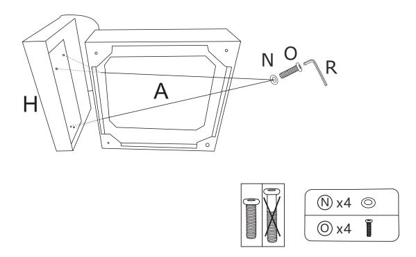
STEP 2: Assemble the Right armrest (I) to the Seat frame (A) with Washers (N) and Bolts (O).
