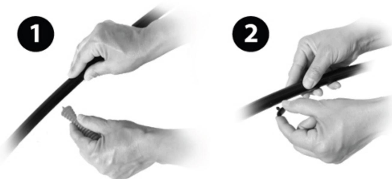
Use the Hole Punch Tool to snap holes in the 1/2in. Poly Tubing.
