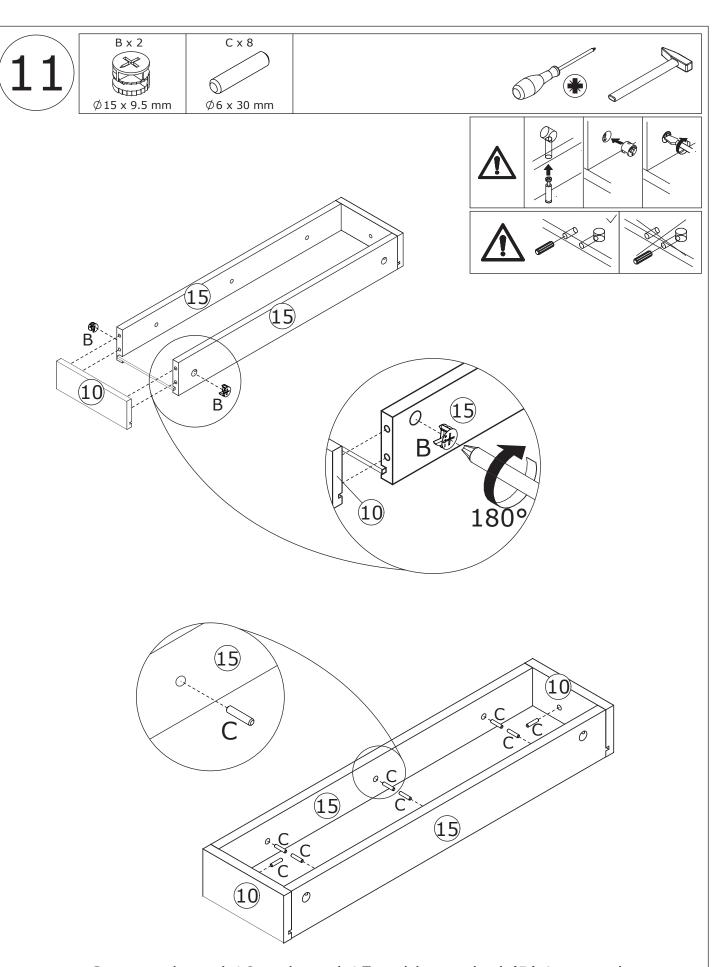
Connect board 10 to board 15, add cam lock(B) into and turn clockwise to tighten as shown. Insert wooden dowel(C) into board 10 and 15 as shown.
