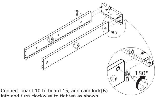
into and turn clockwise to tighten as shown.
