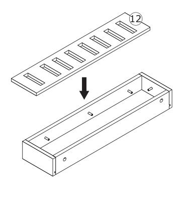
Place board 12 into the part, insert buckle(F) into back slots and fix to tighten as shown.
