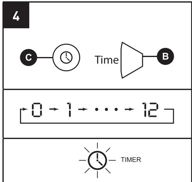
5. To set the timer to power on the heater, first ensure the unit is powered off, then press the timer button on the control panel (C).
