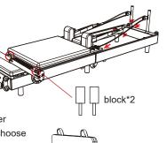
4.Install the block, as shown in the figure, screw the rubber block into the front hole of the skateboard track.You can choose a foot pedal or a Jumpboard according to your personal exercise situation. When installing, insert it into the front groove and turn the plum knob to lock it.
