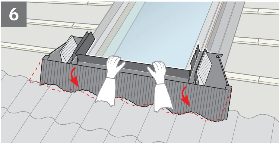
**ENGLISH:** Remove sill flashing section and bend the apron down as shown. This will ensure that the apron lies tightly against the roofing material.
