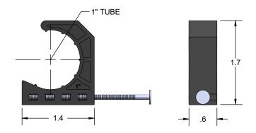
HOLDRITE #191, #192 & #193 Half S-Nail Clamps are ideal for "Surface Mounted" positioning of 1/2", 3/4" & 1" CTS tubing (Copper, CPVC or PEX). The nail is preloaded into the clamp for quick installation. Provides protection against tubing damage caused by abrasion or contact between dissimilar metals.
