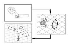
1: Wrapped some teflon tape on the thread of the adapter.
