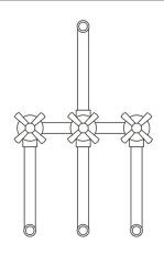
③ Use rubber plug to block the top shower spout, Tub spout connector. Open the water source, check the connection of the upper and lower water pipes, and the pressure of the pipe to ensure no leakage. Make sure there are no water leaks then tilling the wall and install the round decorative cover and the cross handles.
