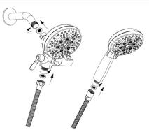
(5) Attach 3 in 1 fixed mount shower head by threading clockwise onto shower arm with rotatable holder to the right and 3-way diverter control handle to the left. Use a wrench to tighten shower head nut to a properly snug fit. Then connect the shower hose to the shower head and hand shower as the pictures shows.
