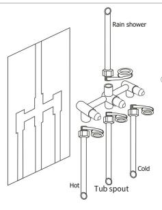
① A.Wrap the pipe tape to the prepared male water pipe and then connecting to the embedded shower valve.Pay attention to the connection of the water inlet and outlet signs.
