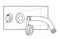
Wrap the shower arm thread with pipe tape before connect to the water pipe.
