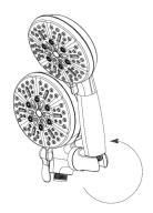
**To Adjust Angle of Hand Shower** Rotate holder in vertical direction to set desired hand shower angle.
