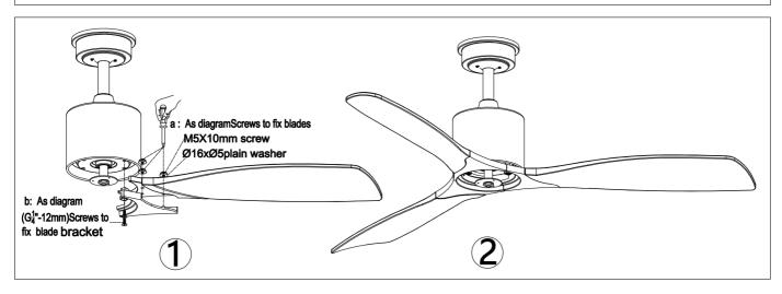
First of all, please refer to step A in diagram 1. Fix blades on connectors by screws, then refer to step B in diagram 1, fix connectors on motor by screws
