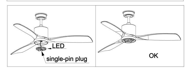
Connect the LED Board to the cables from the lower end of the motor, using the quick splice connector. Then fix the LED board in place onto the metal ring, by means of the magnets.
