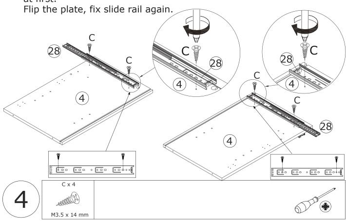
Fix slide rail 28 to plate 6 using screw(C) at first. Filp the plate, fix another slide rail again.
