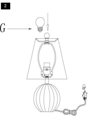
Step 2 Insert the bulb(G) into the socket(C).
