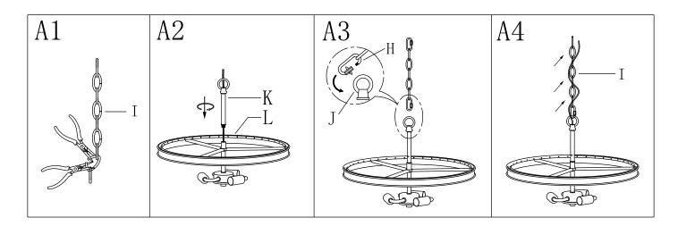
Step A1 » By measuring, determine the correct number of links needed for proper hanging height. Using the chain pliers, disconnect and discard the unwanted part.
