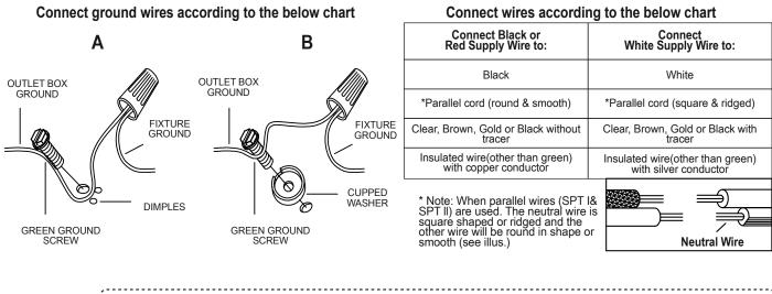
• Twist wires together with plastic wire connectors until tightly joined.
