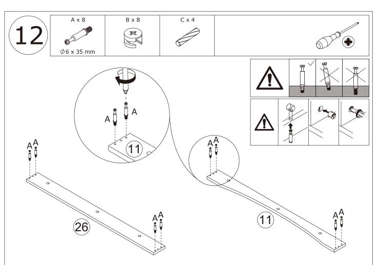
Screw eccentric rod(A) into board 26 and 11 at first. Connect board 12 to board 11 and 26 using wooden dowel(C) at first, add cam lock(B) into board 12 and turn clockwise to tighten as shown.
