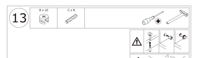
Attach the part to board 9 using wooden dowel(C) at first, add cam lock(B) into board 11,12,26 and turn clockwise to tighten as shown.
