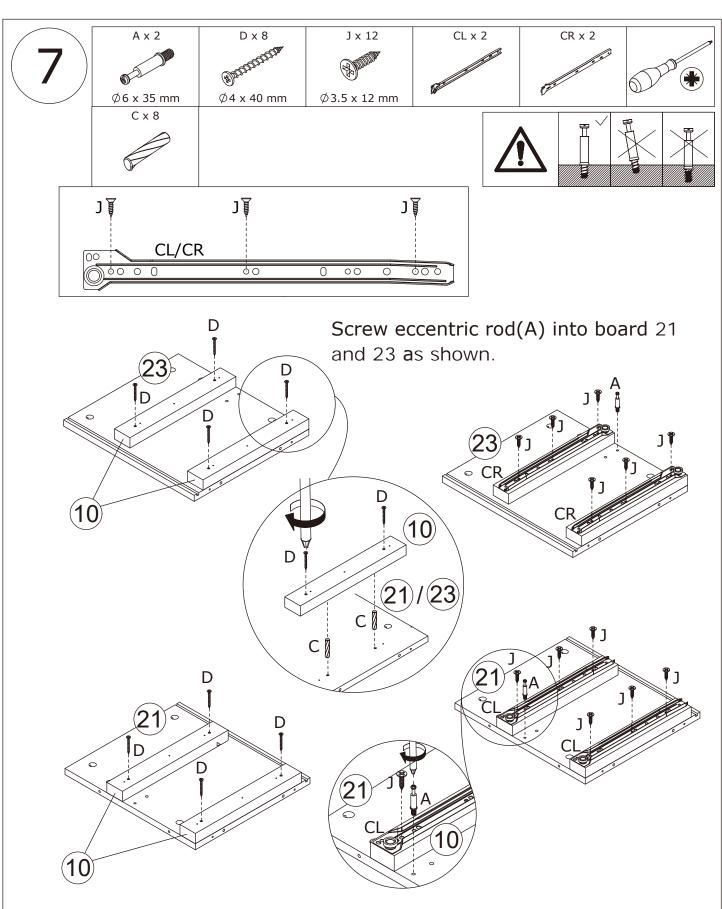
Attach board 10 to board 23 using wooden dowel(C) at first, then fix board 10 to board 23 with screw(D), then fix slide rail(CR) to board 10 with screw(J) as shown. Attach board 10 to board 21 using wooden dowel(C) at first, then fix board 10 to board 21 with screw(D), then fix slide rail(CL) to board 10 with screw(J) as shown.  $\frac{11}{22}$
