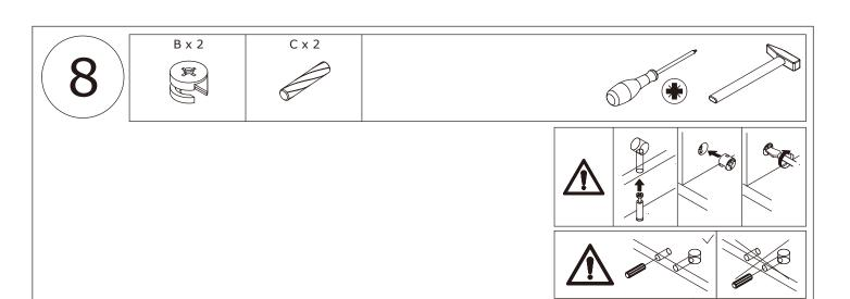
Connect board 13 to board 21 and 23 using wooden dowel(C) at first, add cam lock(B) into board 13 and turn clockwise to tighten as shown.
