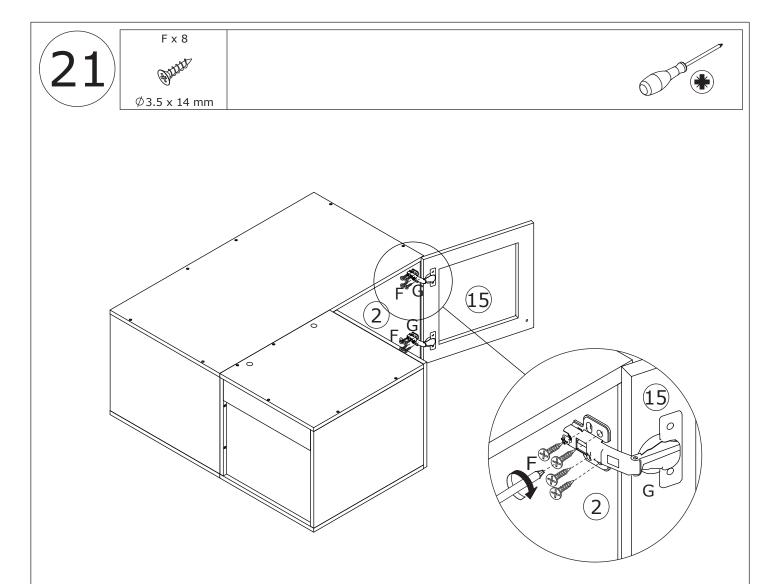
Assemble door 15 to board 2 by fixing hinge with screw(F) as shown.
