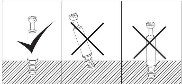
Insert threads of Locking Bolts completely, and stop once threads are no longer visible.
