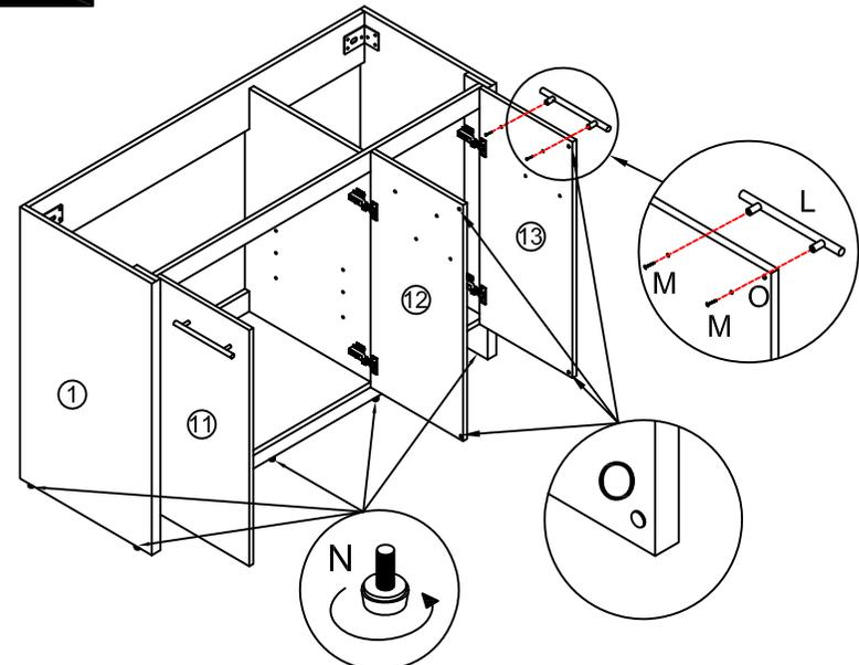
Note: Install and adjust the level screws
