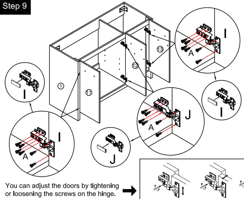
You can adjust the doors by tightening or loosening the screws on the hinge. →
