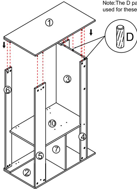
Note: The D parts are used for these two holes
