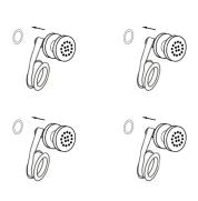
⑥ Wrap some plumber's tape on the body jets thread and screw the body jets to the pipe.
