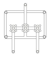
③ Use rubber plug to block the top shower spout, body jet connector. Open the water source, check the connection of the upper and lower water pipes, and the pressure of the pipe to ensure no leakage. Make sure there are no water leaks then tilling the wall and install the round decorative cover and the cross handles.
