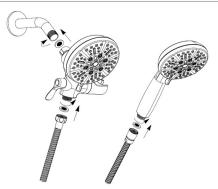
⑤ Attach 3 in 1 fixed mount shower head by threading clockwise onto shower arm with rotatable holder to the right and 3-way diverter control handle to the left. Use a wrench to tighten shower head nut to a properly snug fit.Then connect the shower hose to the shower head and hand shower as the pictures shows.
