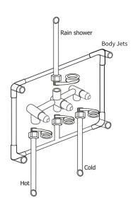
① A.Wrap the pipe tape to the prepared male water pipe and then connecting to the embedded shower valve.Pay attention to the connection of the water inlet and outlet signs.
