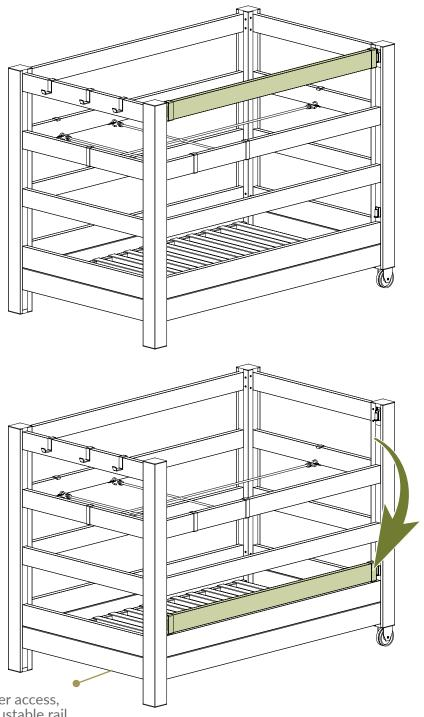
**Tip:** For easier access, place the adjustable rail in the lower position.
