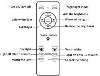
1. The remote control is mainly for the ceiling lights and panel lights currently on sale which are dimmable and color changeable.
