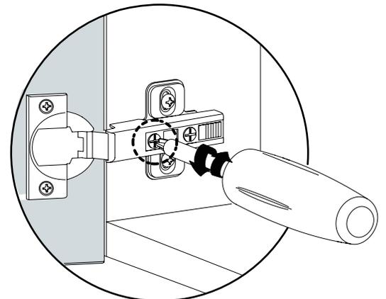
**1 REMOVE THE SIDE MOUNTED BRACKET / RETIRAR EL SOPORTE LATERAL**
