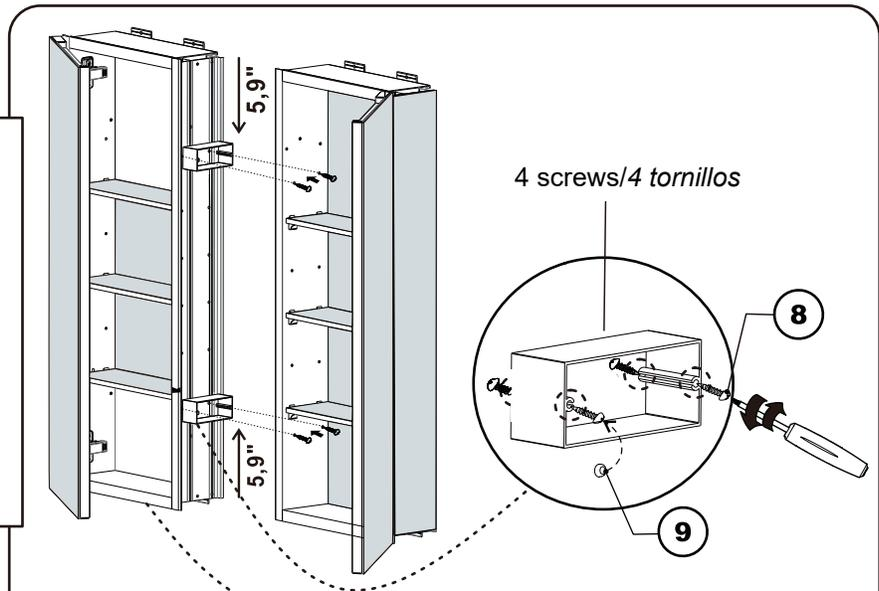
For two cabinets, install 2 connectors; for three cabinets, install 4 connectors.
