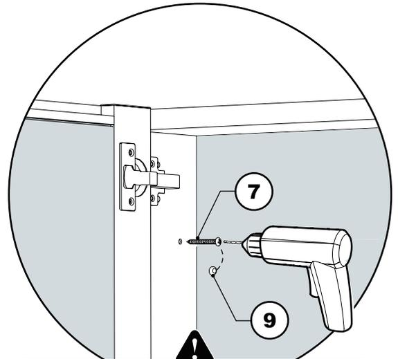
**DON'T TIGHTEN THE SCREW WITH A DRILL. TIGHTEN THE SCREW MANUALLY**
