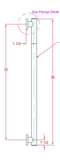
1-1/4" x 18ga. S.S. Round Tubing formed to eliptical shape of 1-1/2" x 1"
