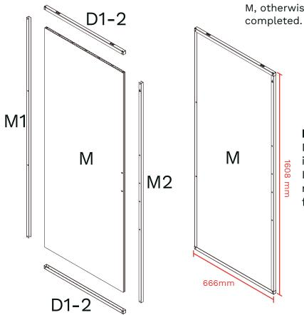
**Note:** M1/M2 need to be installed securely with part M, otherwise, the subsequent steps cannot be completed.
