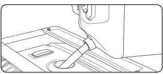
6. Screw on the fuel cap and wipe away any spilled fuel.
