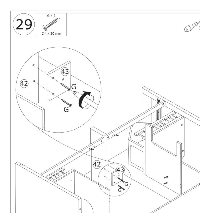
Fix panel 43 to panel 42 with screw(G) as shown.
