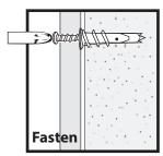
place screw through drill hole and tighten into anchor
