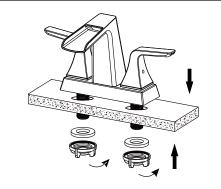
1.Please confirm the two holes on the basin are through holes as shown from the instructions before install.First, remove all fixing sets from the fixed group, and then put the body through the hole on the basin, assemble all fixing sets to the body.
