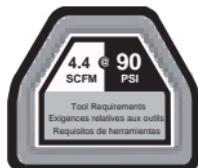
**IMPORTANT:** To operate correctly, this tool requires airflow that is at least 4.4 cubic feet per minute (SCFM) at 90 pounds per square inch (PSI). Check the specifications of your air compressor to be sure that it can support both the minimum SCFM and PSI required. The air hose length could affect how much air pressure the tool is actually receiving. You may need to adjust the air pressure higher on the air regulator to achieve the required 90 PSI.
