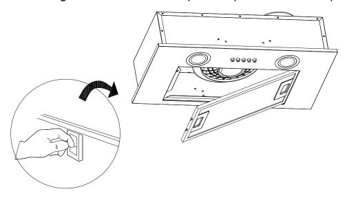
2. Push the LED lamp holder out from the cabinet by hand, or use slotted screwdriver to prize up the LED lamp around the edges, pull out the LED lamp and the wire together.
