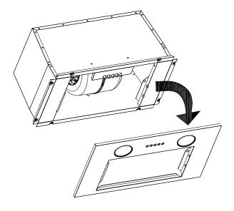
7) Put the range hood into the cabinet that have been drilled holes, then fix the range hood on the cabinet by 8 pcs of 0.16\*0.79 screws.
