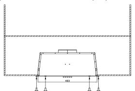
8) Insert the plug of LED light into the power protection box and close the cover. Then install the front panel and drill 2 pieces of setscrews.
