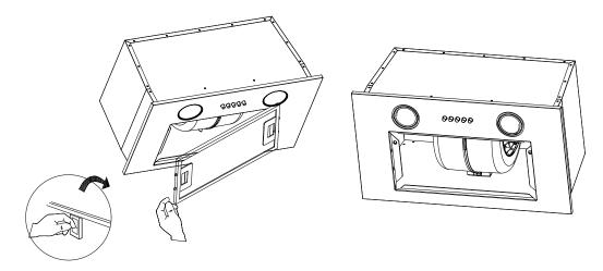
2. Place the carbon filter into the unit and turn it in the clockwise direction to lock it in place.
