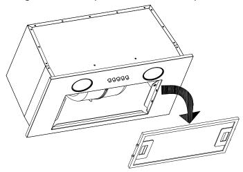
5) Loosen the two screws of the front panel, pull down the front panel and pull out the lamp line. Open the power protection cover and disconnect the plug.
