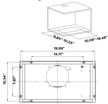
3) Drill holes on the corresponding positions in the cabinet according to the below picture.
