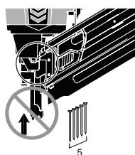
This tool is equipped with a lock-out feature. When approximately 5 nails (depending on nail size) remain in the magazine, the workpiece contact (safety element) will be locked in the undepressed position until more nails are loaded into the magazine and the feedershoe is pulled back.
