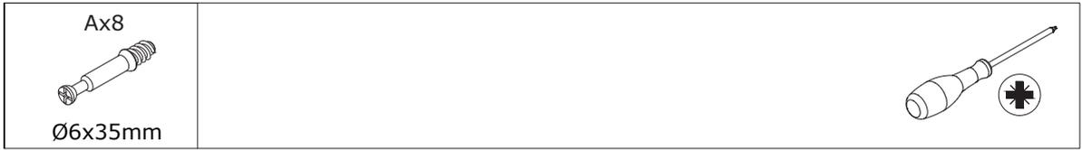
Insert quickfit screw(A) into corresponding holes in plate 8 and 9 with a screwdriver as shown.
