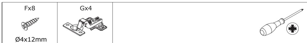
Fix hinge(G) to plate 12 and 13 using screw(F) as shown.
