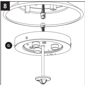
9. Align the two key slots in the light kit (Q) with the two previously loosened light pan screws (S). Place the light kit (Q) over the two screws and turn the light kit (Q) clockwise. Re-install the previously removed light pan screw (S) and tighten all three screws securely.
