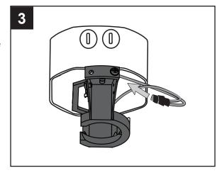
Align the canopy (E) over the loose mounting bracket screws (M) preassembled on mounting bracket (D). Place the keyholes of the canopy (E) onto the mounting bracket screws (M) and rotate the canopy (E) clockwise.
