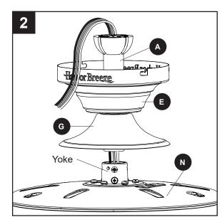
3. Slide the downrod (A) into the yoke of the motor assembly (N), align the holes, then re-install the downrod pin (B) and downrod clip (C). Secure with set screws (L).
