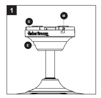
2. Secure the canopy (E) with the mounting bracket screws (M) previously removed (Step 4, page 8). Tighten all mounting bracket screws (M) securely.
