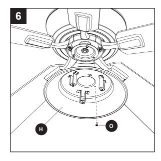
7. Remove one light pan screw (S) from one of the three brackets below the light pan (H) and save. Loosen but do not remove the other two screws on the other two brackets.
