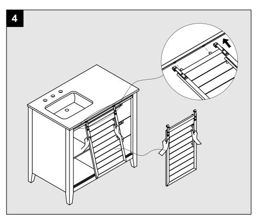
Note: In case replacing the slider sub-assembly, untighten the bolts with Allen wrench (not included).
