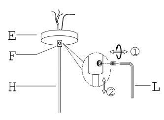
5 » If needed, shorten the extra length of the fixture wires from cord (H) so that they all are at least 6 inches (152.4 mm) long above canopy (E) within the outlet box.
