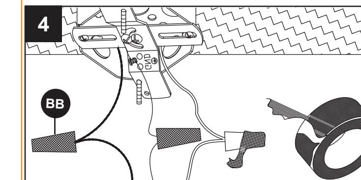
**!** Attach BB to connections with electrical tape (not included).
