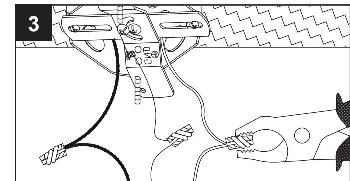
**!** Feed wires. Twist stripped wire ends together with pliers (not included), black to black, white to white, and ground/bare to ground/bare.
