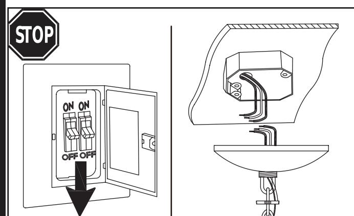
**! Turn off the power and remove existing fixture.**
