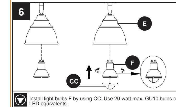
**!** Install light bulbs F by using CC. Use 20-watt max. GU10 bulbs or LED equivalents.
