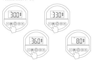
5. Use the "+" and "-" buttons to set the desired pressure. Use the tire pressure guide on the inside of the driver's door for guidance.
