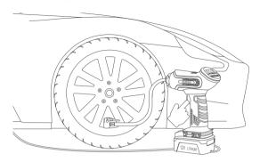
8. After inflation, press and hold the Power Button for 3 seconds to turn off the tire inflator.
