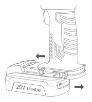
Hold the handle and press the button above the battery to remove the battery.
