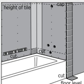
On walls where tile will reach the floor, determine whether floor is level by measuring distance to desired tile height on both sides of area to be tiled. If there is a difference (e.g., the floor is lower on one side), lay one vertical row of tile from highest point down to floor. Affix tiles with dabs of mastic.
