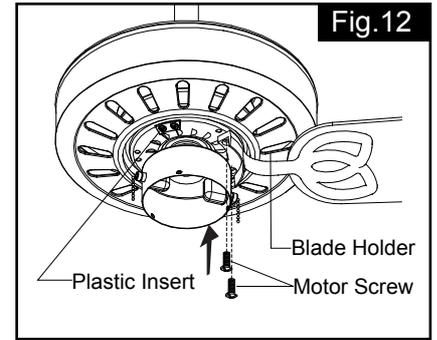
Secure blade holders to the motor with motor screws and washers.
