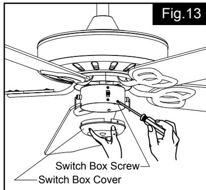
Make sure the wires of the fan light in the switch box are capped with wire nuts. Secure the switch box cover with the switch box screws.
