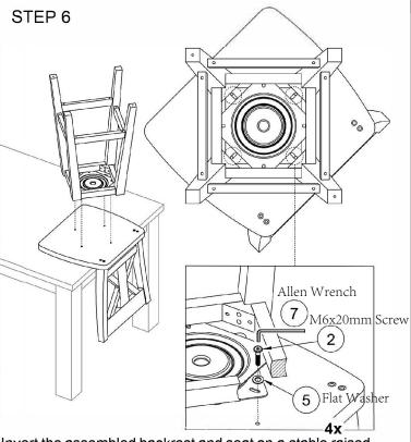
Invert the assembled backrest and seat on a stable raised surface such as a table. Attach the Swivel Plate located on the Apron with Swivel Plate (Part E) to the Seat using (4) M6x20mm Hex Screws (Part 2) and (4) Flat Washers (Part 5) Tighten all screws using the Allen Wrench (Part 7). Return Chair to the upright position.
