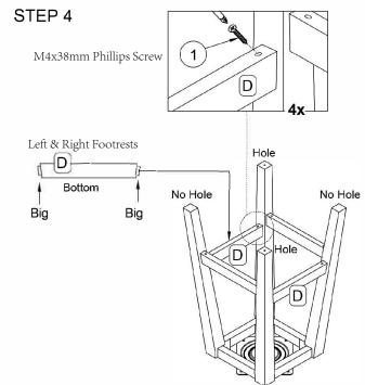
Attach Left & Right Footrests (Part D) to the large holes on the Chair Legs (F & G) using (4) M4x38mm Phillips Screws (Part 1). Tighten loosely with Phillips Screwdriver (Not Included).
