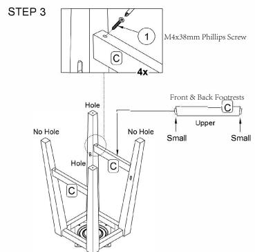
Attach Front & Back Footrests (Part C) to the small holes on the Chair Legs (F & G) using (4) M4x38mm Phillips Screws (Part 1). Tighten loosely with Phillips Screwdriver (Not Included).
