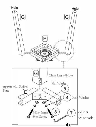
Attach (2) Chair Legs with Hole (Part G) on opposite sides of the Apron with Swivel Plate (Part E), using (4) M6x45mm Hex Screws(Part 3), (4) Lock Washers, (Part 4) and (4) Flat Washers (Part 5). Loosely tighten with Allen Wrench (Part 7).
