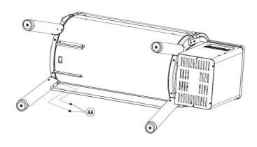
6.Attach the Front Plate (23) on Rear Leg (20) and Front Leg (21) by using the Screws (AA). The two positions are installed in the same manner, as shown.
