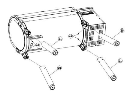
5.Attach the Back Plate (22) on Rear Leg (20) and Front Leg (21) by using the Screws (AA). The two positions are installed in the same manner, as shown. Use Screwdriver (FF) to tighten them.
