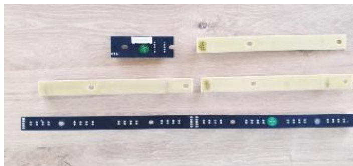
Photo 120 - Lamp PCB, receive PCB view of model S230C
