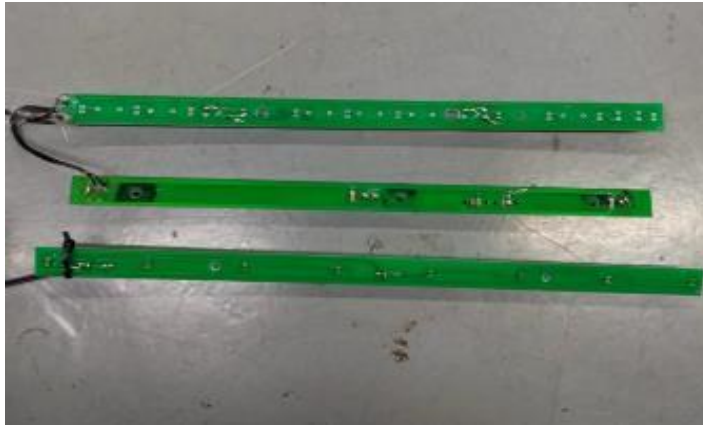
Photo 148 - Lamp PCB view of model C280
