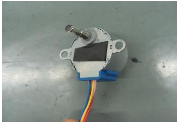
Photo 63 - swing motor view of model RFI-3901LA
