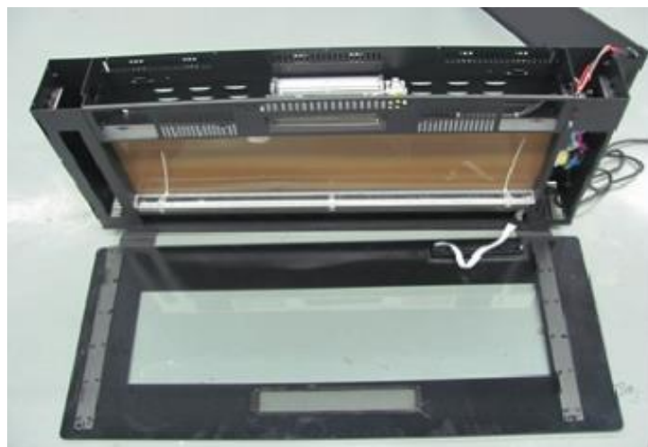
Photo 72 - internal view of model RFH-4201LA
