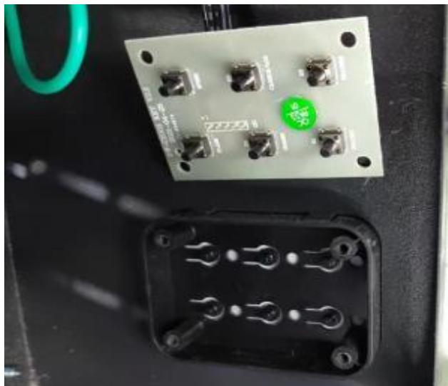
Photo 141 - Control PCB view of model L250, C280
