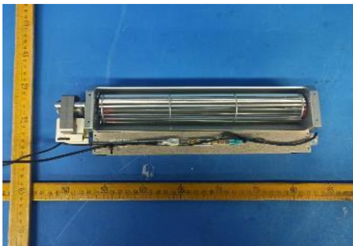
Photo 86 - internal view of model RFH-3001L with optional heating element assembly (as representative RFH-3001LA, RFH-3601LA, RFH-4201LA, RFH-5001LA, RFH-6001LA, RFH-7401LA, RFH-10201LA are same except shape size).
