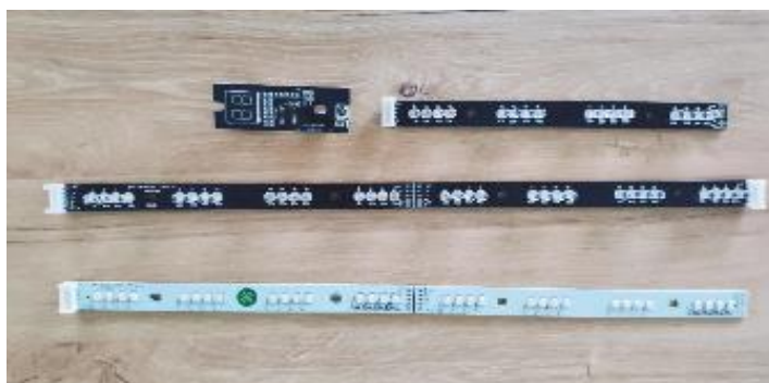
Photo 122 - Lamp PCB, receive PCB view of model S230C
