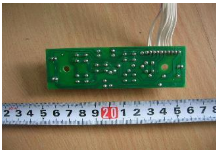
Photo 16 - control PCB of model ZBI-15SRLT/R16
