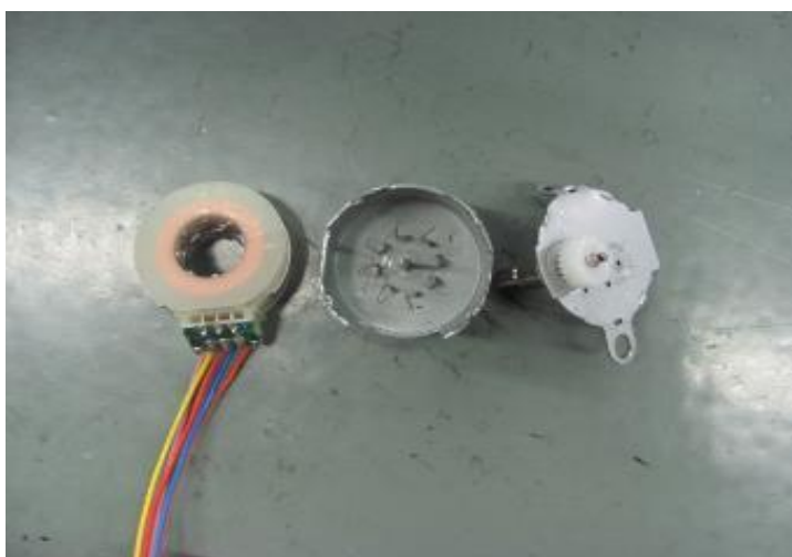
Photo 63 - swing motor view of model RFI-3901LA
