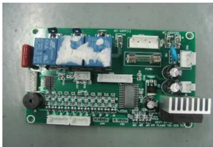
Photo 78 - power PCB view of model RFH-4201LA
