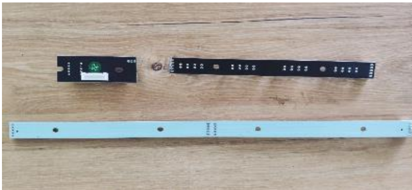
Photo 101 - Lamp PCB, receive PCB view of model S180
