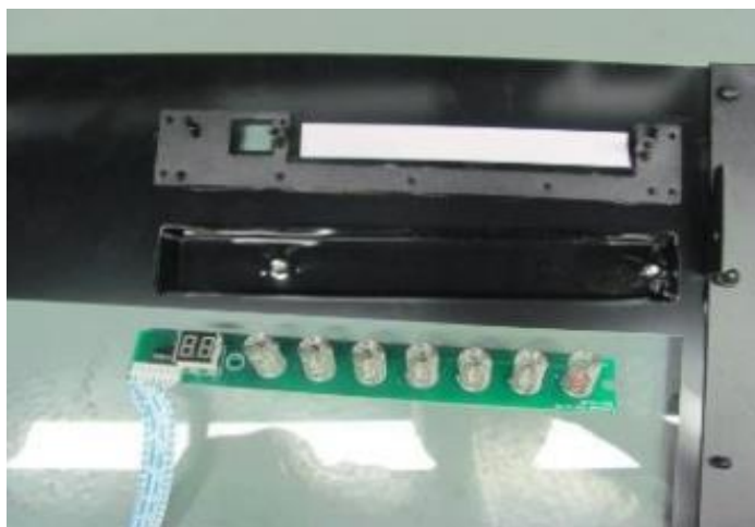
Photo 74 - control PCB view of model RFH-4201LA
