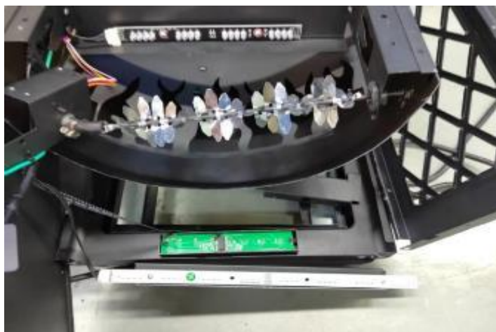
Photo 98 - Power PCB view of model S180, S230B, S280
