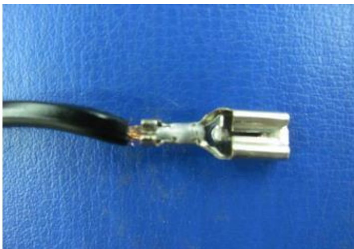
Photo 82 - connection view of supply cord to internal wiring for all models
