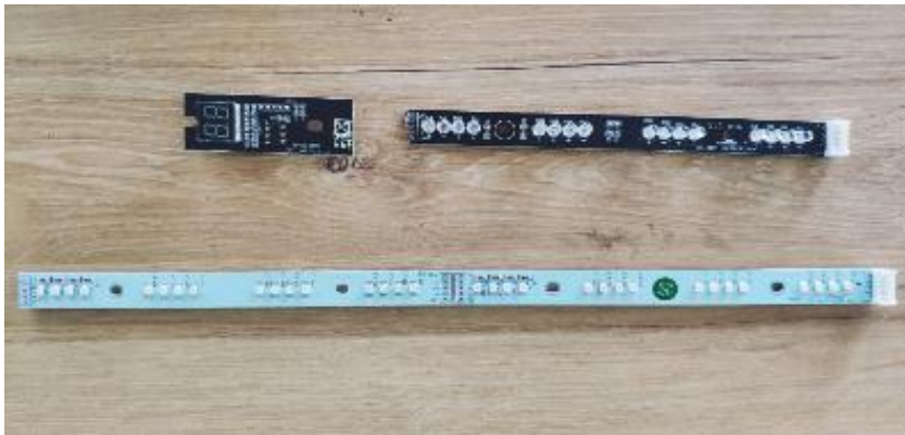
Photo 100 - Lamp PCB, receive PCB view of model S180
