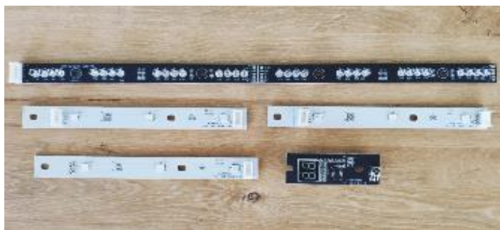
Photo 120 - Lamp PCB, receive PCB view of model S230C
