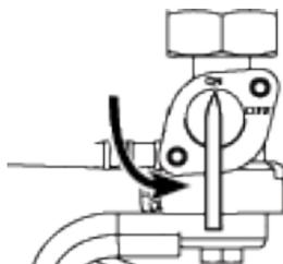
**Note:** If cold starting, move the choke lever to the ON position.
