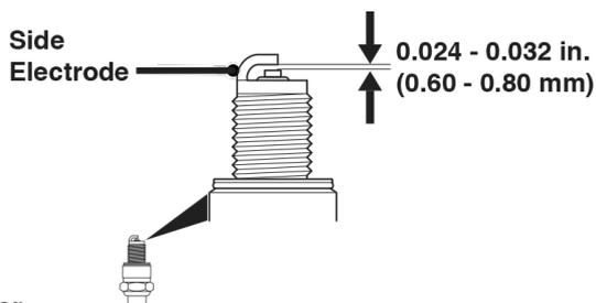
7. Carefully install the spark plug finger tight, then tighten as additional 3/8 to 1/2 turn with the spark plug wrench.
