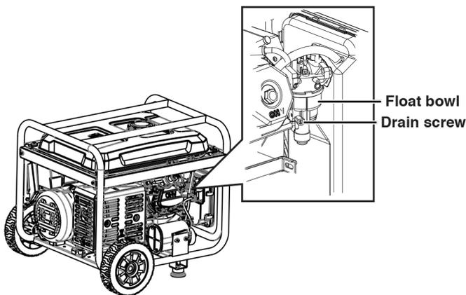
3. Place an appropriate gasoline container under the drain screw to catch the drained fuel.
