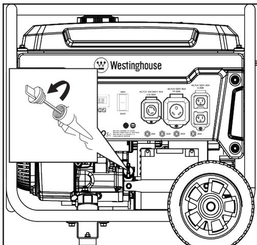
4. Insert the dipstick into the oil filler neck without screwing it in. Remove the dipstick and verify that the oil level is within safe operating range between the low (L) and high (H) marks on the dipstick.
