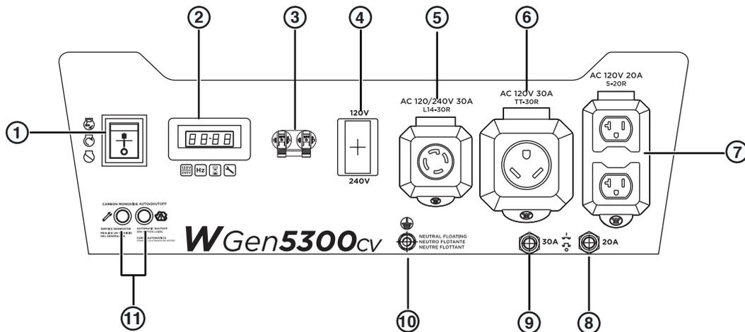
1. **Run/Stop Switch:** Push to Run position to start or Stop position to shut the generator off.
