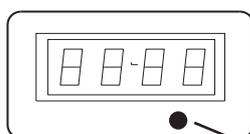
Push the Mode button to cycle through the data display modes.
