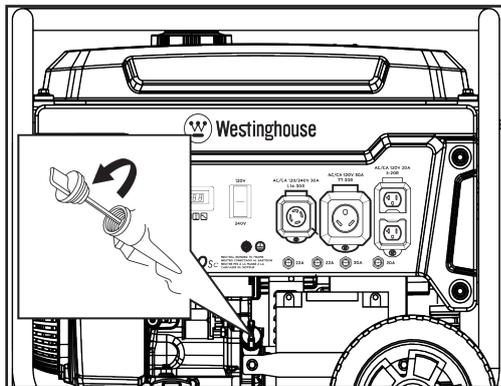
2. Using the supplied funnel and oil, add oil into oil filler neck.
