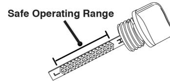
5. If low, add recommended engine oil incrementally and recheck until the level is between the L and H marks on the dipstick. **DO NOT** overfill. If over the H mark on the dipstick, drain the oil to reduce the oil level to the full mark.
