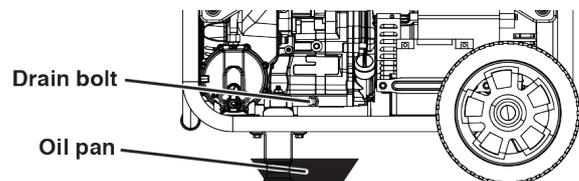
5. Install the oil drain bolt and tighten securely.
