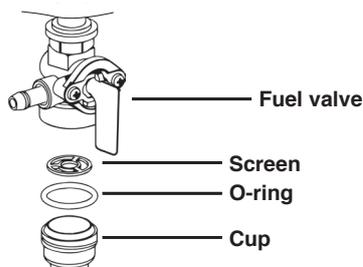
4. Wash the sediment cup, o-ring, and screen in a nonflammable solvent. Dry thoroughly.
