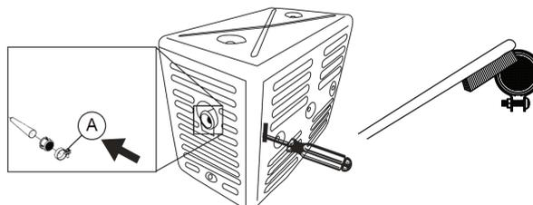
3. Carefully remove the carbon deposits from the spark arrestor screen with a wire brush. The spark arrestor must be free of breaks and tears. Replace the spark arrestor if damaged.
