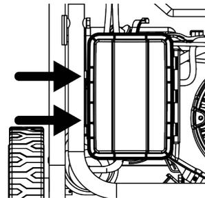
3. Clean the air filter with compressed air. Replace if damaged.
