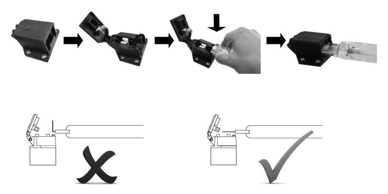
**ATTENTION:** Please make sure the wire of the lamp is straight when you install the lamp. If not, the lamp will not connect securely with the socket.
