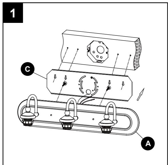
2. Using a 5/16 in. drill bit (not included), drill pilot holes at marked locations. For masonry installations, insert wall anchors (EE) into the holes. Otherwise, attach backplate (C) to wall using machine screws (DD) and use mounting screws (CC) to secure it to the outlet box. **Note:** Make sure the narrow end of the keyhole slots on backplate (C) slide down over the screw heads.
