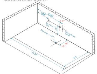
The safe distance between power supply and water supply should be not less than 30cm
