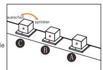
C Waterfall/Sprinkler transferable switch(Marked with Icon) B Controls the water inflow and the water temperature. Up the handle to open, otherwise down the handle to close water inflow (You pull up the handle higher; the water force will be stronger. Otherwise, the water force
