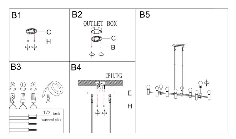
Step B1 » Unscrew canopy nuts (H) from the canopy (E) and then remove the mounting plate (C).
